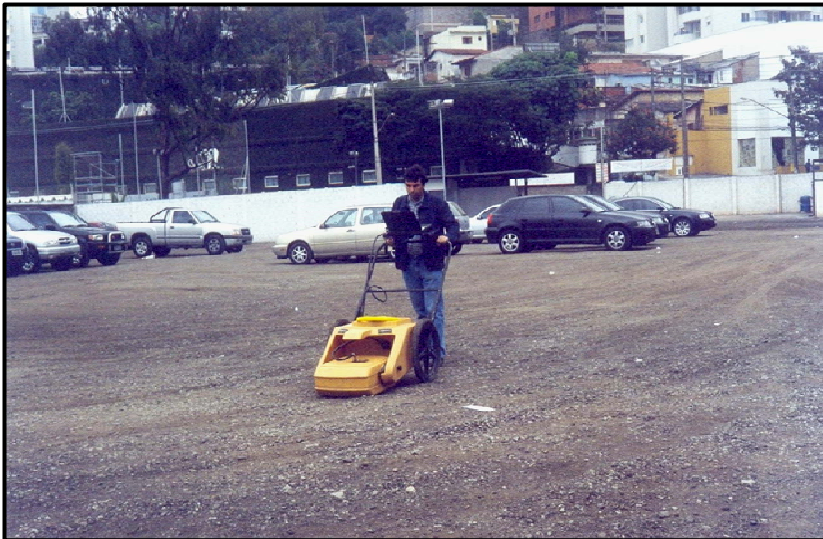
Ground Penetrating Radar - GPR
