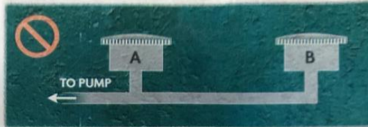
Illustration A: These drains have been placed in series, with the tee set under Drain A. The drains can't pull equally. Drain B is weaker. If Drain A were to become blocked, its counterpart may not be able to prevent a vacuum from forming.
