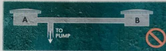
Illustration B: Here, the tee is set too close to Drain A and too far from Drain B. Again, Drain B becomes less effective.
